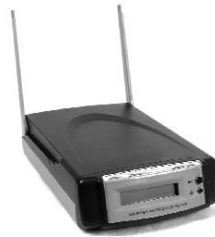
Wireless network server
