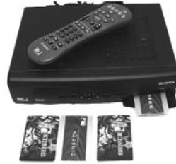
Satellite audio, video receiver, and access cards
