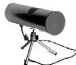
Directional antenna for wireless card
