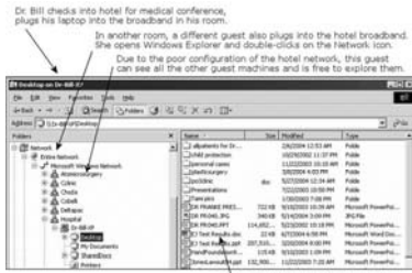
This is an actual screenshot taken at a five star hotel in Boston but to protect privacy we changed the names of computers, folders, and files. Note that no hacking tools were required to see or to access Dr. Bill's files. CSH5 Figure 15.2 Poorly configured hotel room Internet connectivity
