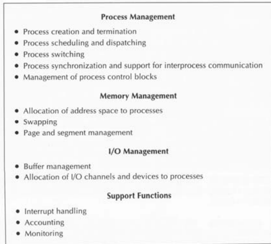
Exhibit 24.3 Typical Kernel Mode Operating System Functions
